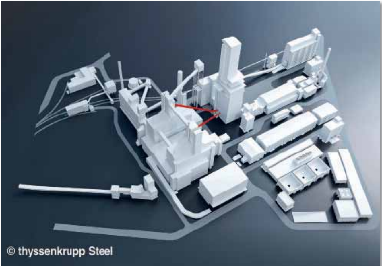
Fig 2 Schematic of the proposed DRI plant in Duisburg with the conveyors shown in red (©thyssenkrupp Steel Europe AG)
