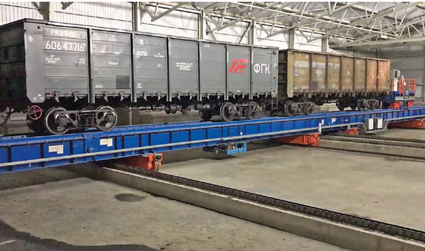
SCHADE Triple Wagon Traverser with on-board Wagon Ejector
