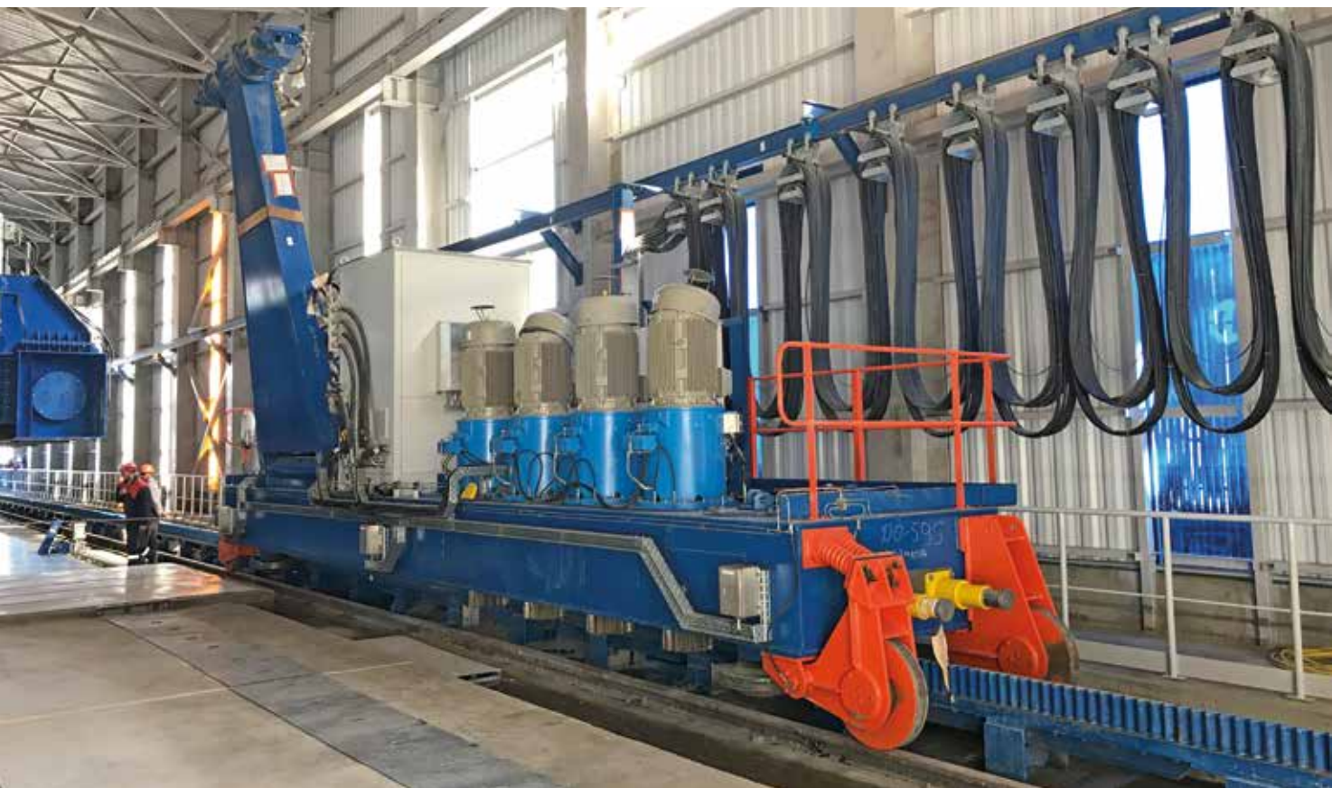
SCHADE Wagon Charger with integral spine bar and cable festoon
