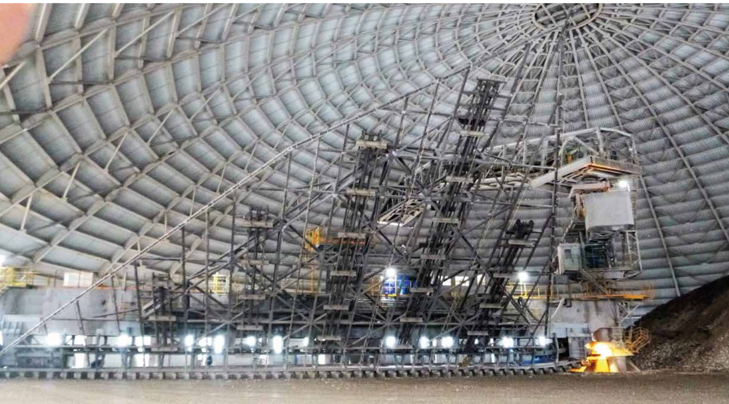
Innovation by SCHADE: Active Harrow System on a Bridge Type Reclaimer
