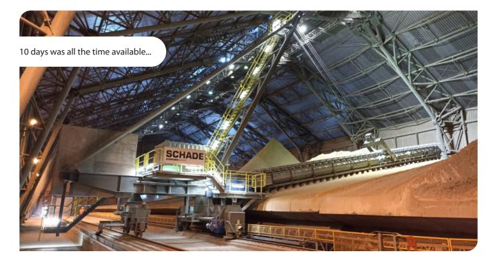
A 200t/hr reclaimer at a cement plant in Górażdże, Poland had been in operation for many decades. It was due to be replaced with a SCHADE Cantilever Reclaimer, plus an associated Belt Conveyor, with the conveying capacity doubled to 400t/hr. SCHADE, part of AUMUND Group, was responsible for the engineering, design, fabrication and supply. With the support of AU-MUND Group Field Service the installation was supervised and the machines were commissioned within an extremely tight time-frame.
