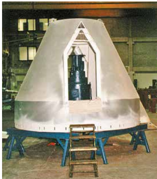
Assembled CTX-IV 5000, view into the support/maintenance arm, onto the planetary drive unit
