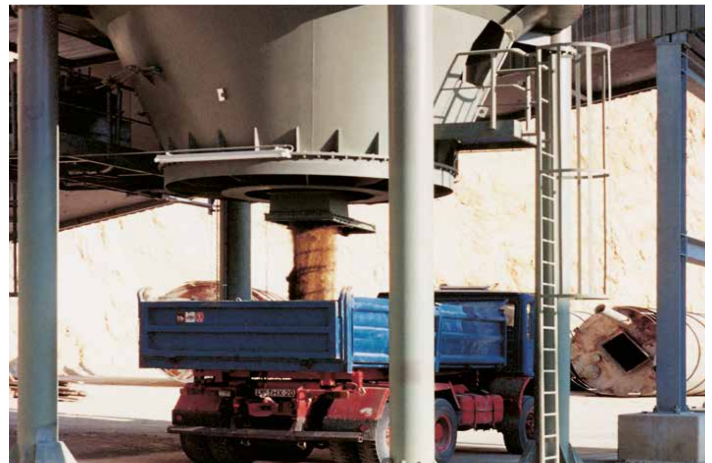
CENTREX® CTX-IV with internal drive. Discharge from a steel plate silo with truck loading
