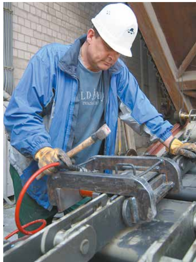
Pre-assembly of chain strands
