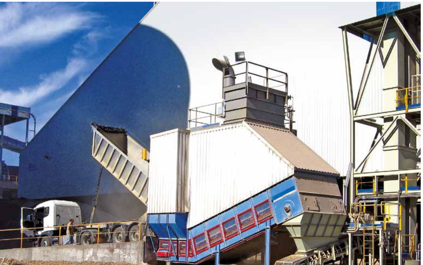
The Samson® MF with deflected chassis and full enclosure including dust filter receives cement clinker
