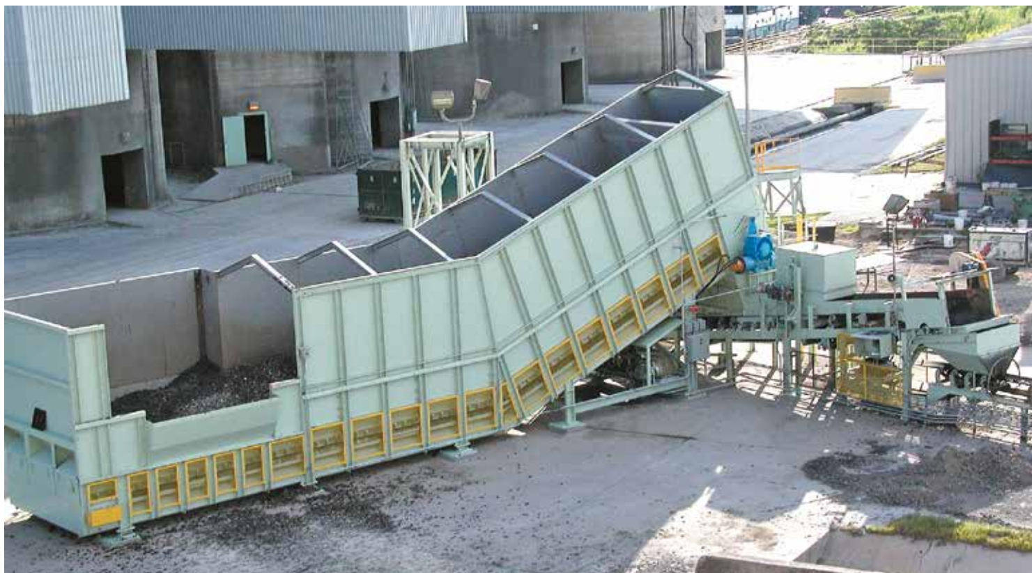
The Samson® MF800 series provides 100 cubic metres of live storage for alternative fuels in a Cement Plant
