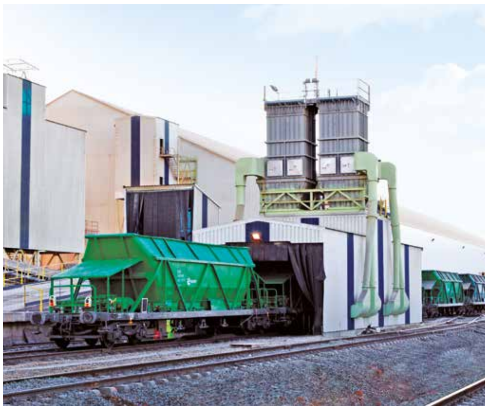
Discharge facility for hopper bottom railcars receives coal for a Cement Plant including a Samson® MF with 80 tons holding capacity
