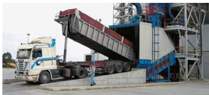
Samson® MF clinker intake for cement grinding plant with integrated dust extraction
