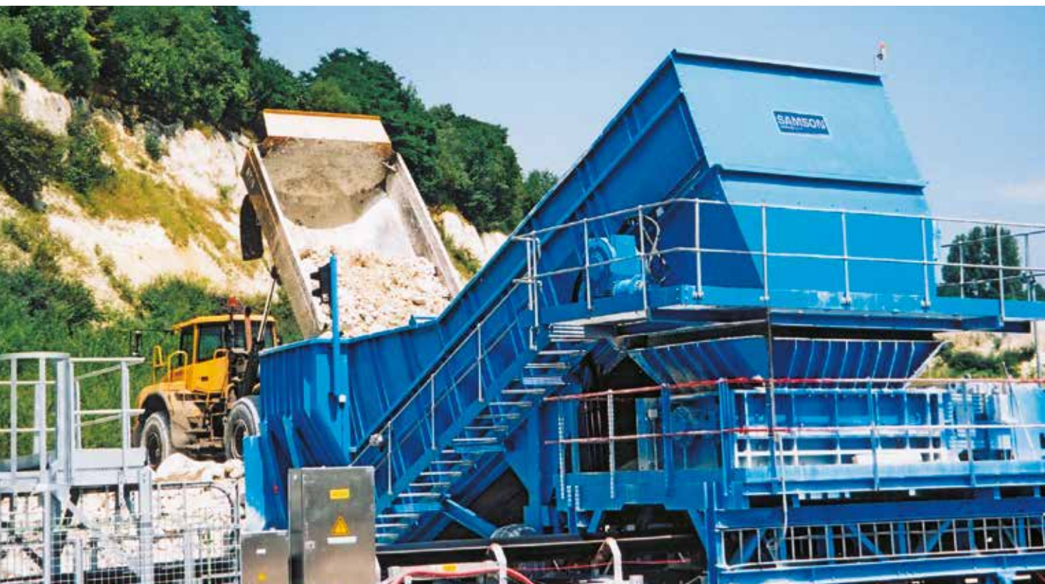
Samson® MF plus Twin Shaft Rotary Sizer receives as-mined limestone from dump trucks and provides a manageable lump size for onward conveying
