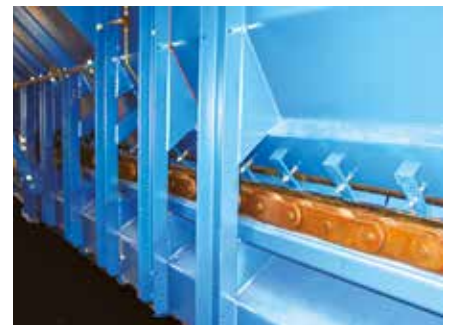
External chains outside the material flow
