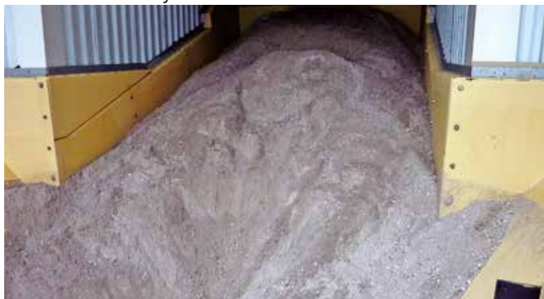
Samson® MF raised discharge permits transfer direct to surface mounted belt conveyor
