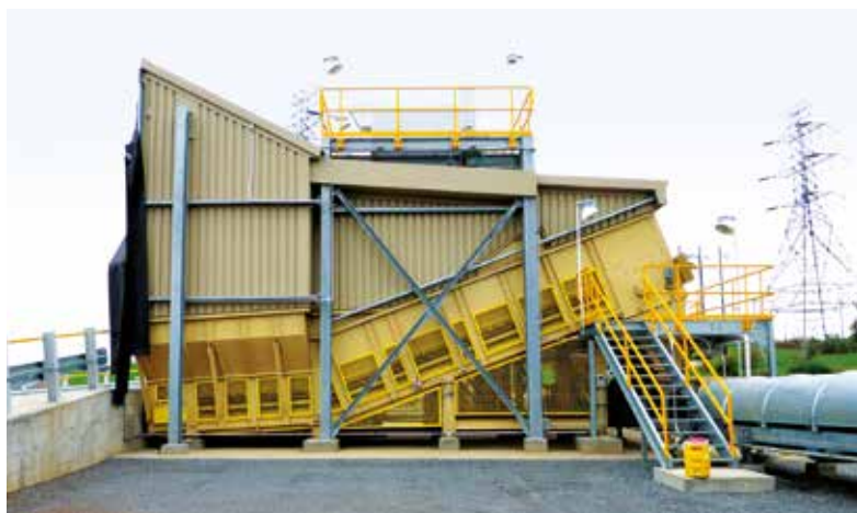
Samson® MF raised discharge permits transfer direct to surface mounted belt conveyor
