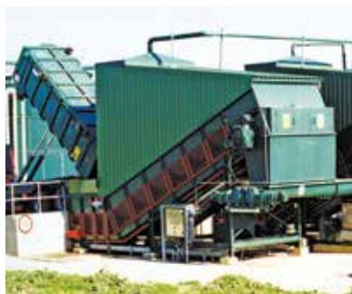
Enclosure with fume extraction for odious materials
