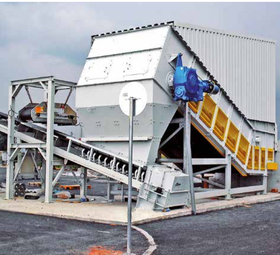
Samson® MF with teaser discharges to an inclined belt conveyor
