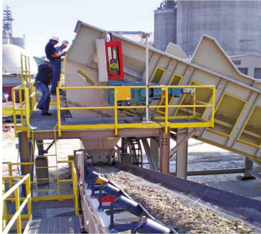
Samson® MF1600 with tandem drives using two helical/bevel speed reducers mounted one each side of the extended head shaft
