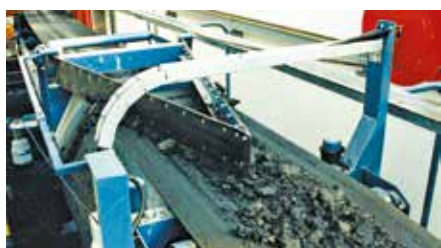
The Samson® MF horizontal storage bunker with overhead conveyor and plough discharger
