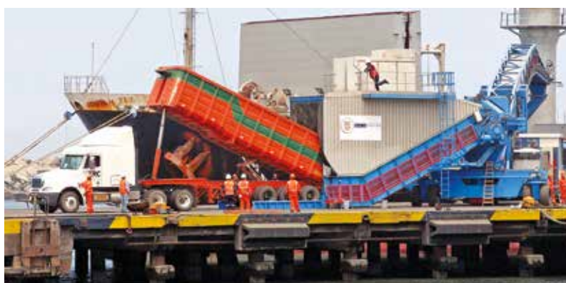
Samson® MF integrated to a Mobile Shiploader receives copper and gold concentrate
