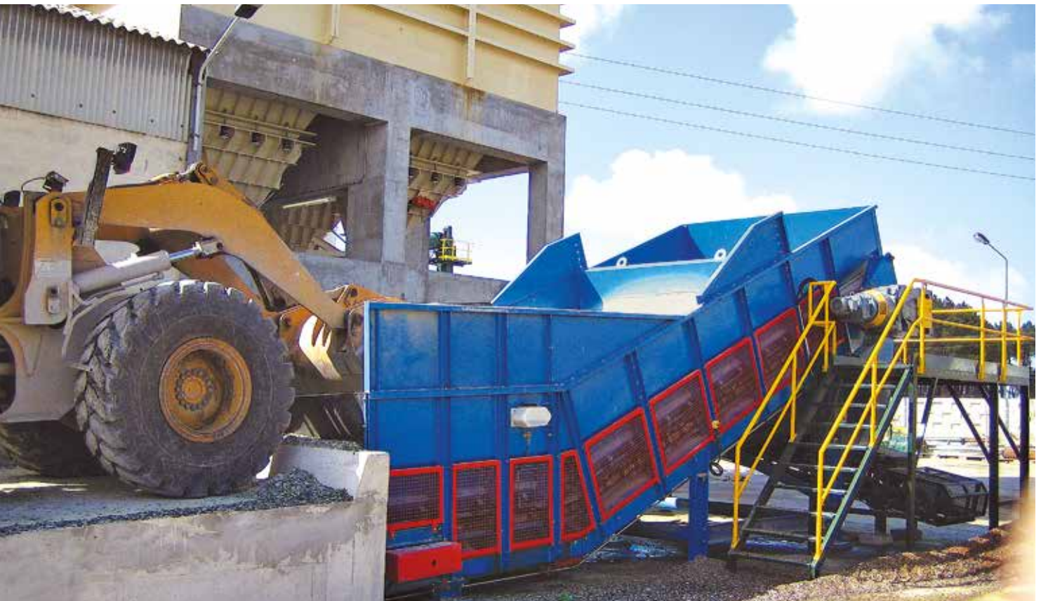
The Samson® MF with deflected chassis and parallel entry (width 3.0 m) receives broken glass from both tipping trucks and shovels
