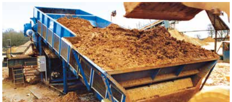
The Samson® MF with Straight Chassis and flared entry (width 4.5 m) receives sandy clay from shovels
