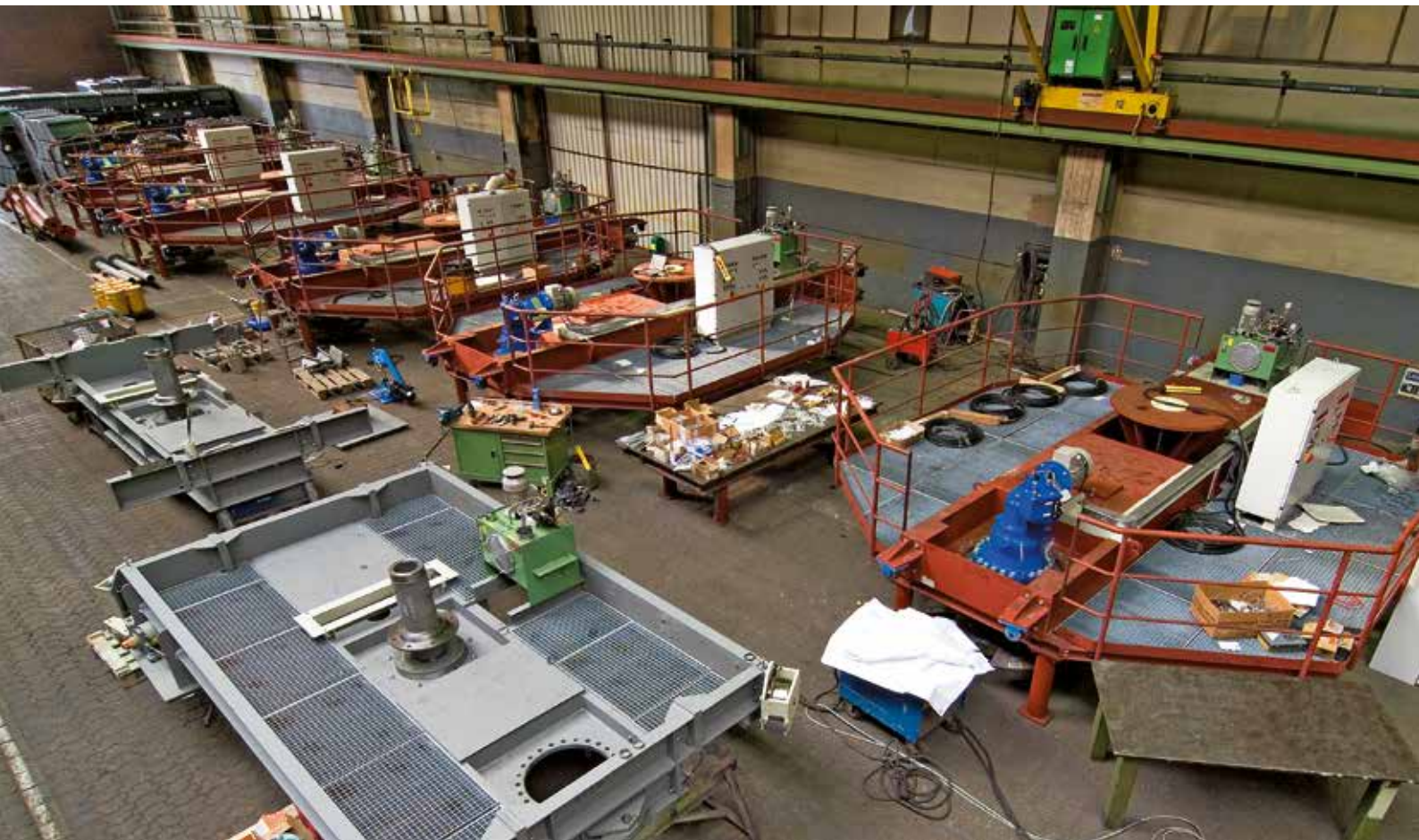
5 BEW-K's 10,000/4,500 during assembly in the workshop at Rheinberg, Germany
