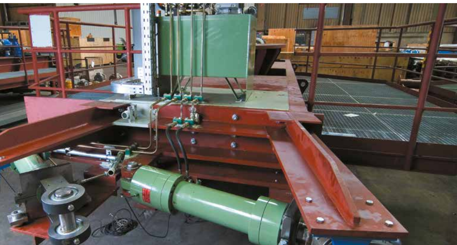
Chassis of BEW-K, view onto hydraulic cylinders for rotation
