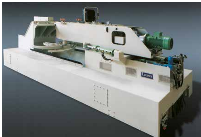
AUMUND Rotary Discharge Machine type LOUISE BEW with single sided discharge and double swivel mechanism
