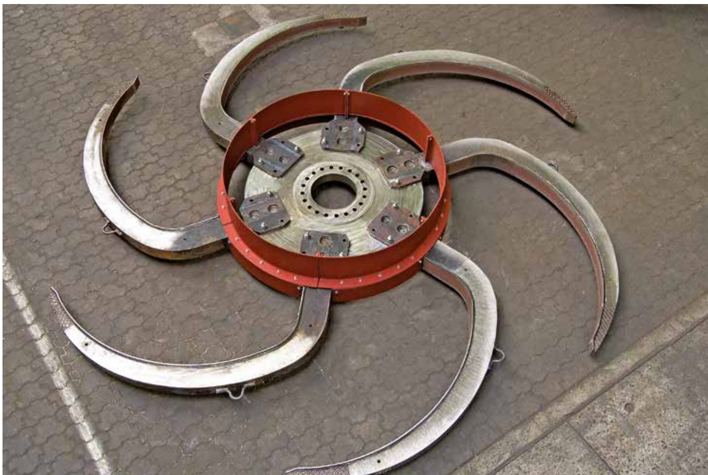
BEW-K discharge wheel, \varnothing 4,500 mm
