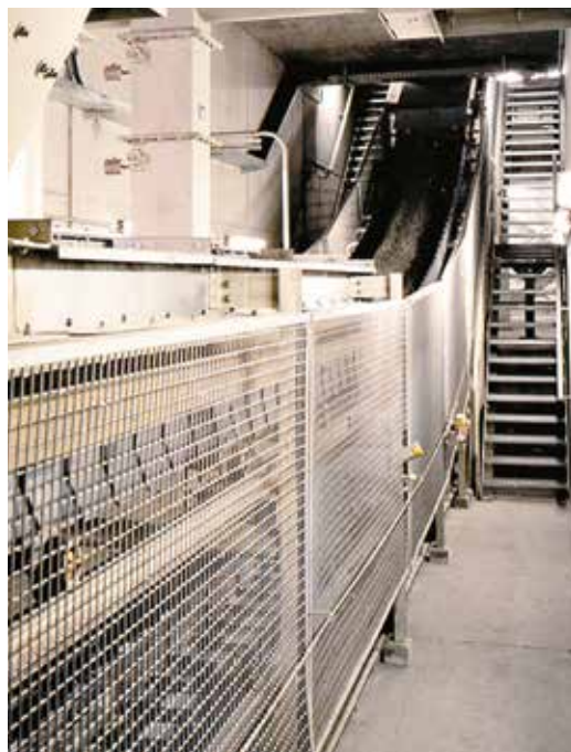
Deep Drawn Pan Conveyor under Clinker Cooler
