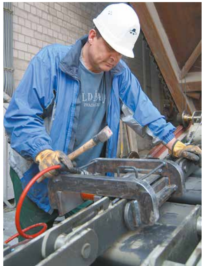
Pre-assembly of chain strands
