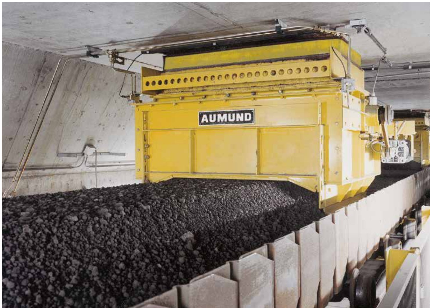
AUMUND Silo Discharge with Remote Control (example)
