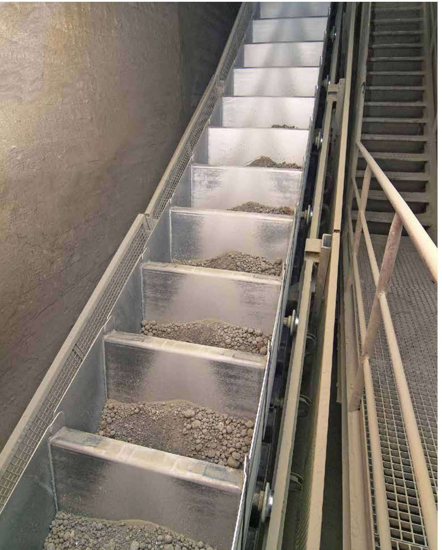
Clinker Transport with AUMUND Conveyor type BZB
