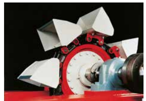
Chain Bucket Elevator
