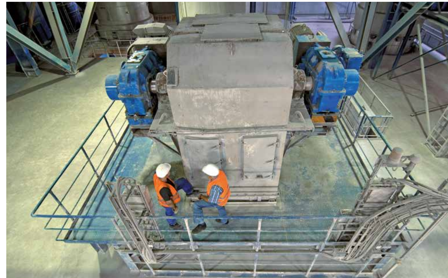
Head of Double Bucket Elevator with double drive and two bucket strands
