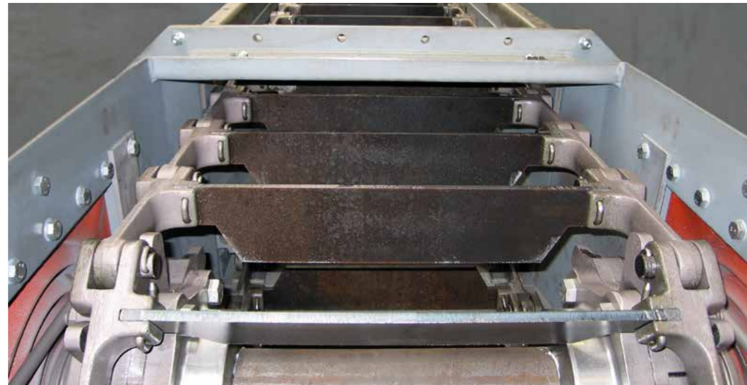
Troughed chain conveyor handling alumina, lime or filter dust
