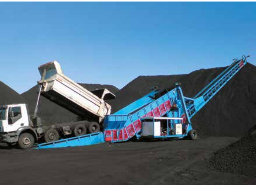
Material intake with SAMSON Material Feeder and stockpiling with Stormajor®
