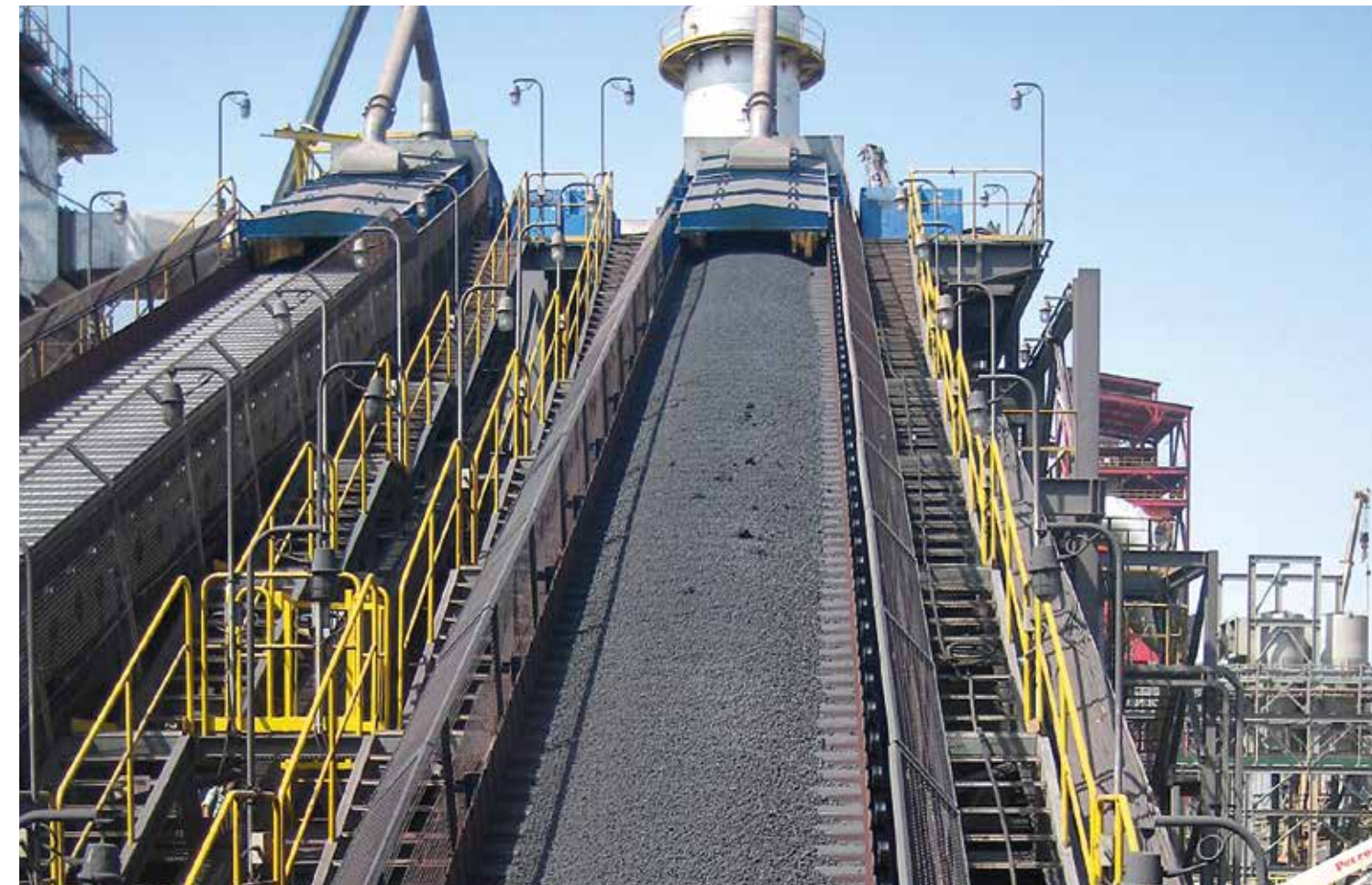
AUMUND Conveyor after Annular cooler for hot pellets
