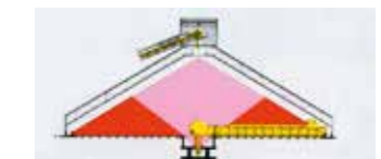
Covered stockpile with MOLEX® without central column
