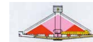
Covered stockpile with MOLEX® and central column
