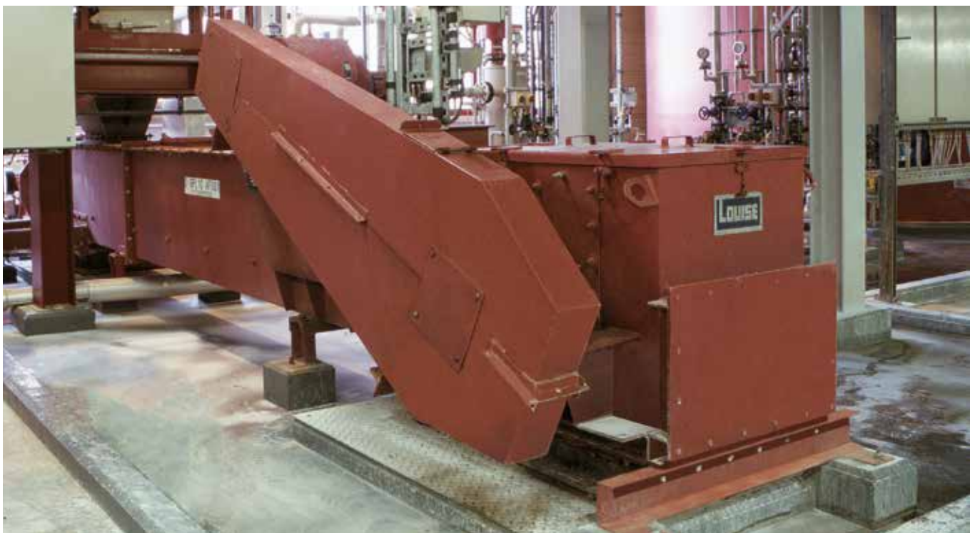
A double-strand Chain Conveyor loads FGD Gypsum from the flue-gas desulphurisation into the storage silo
