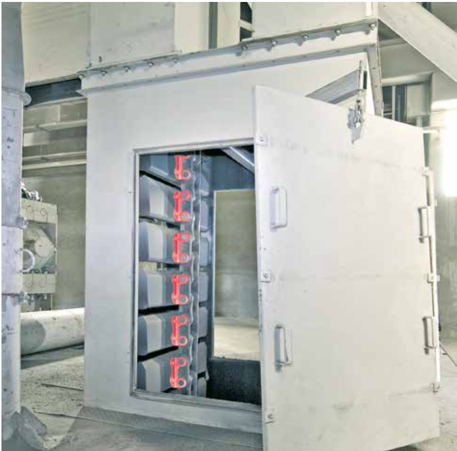
Assembly casing with hinge-supported door for easy maintenance
