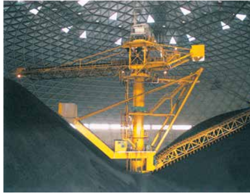
Pet-Coke intake facility with onward transport by belt conveyors to SCHADE storage
