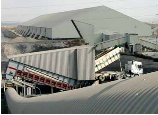
Pet-Coke intake facility with onward transport by belt conveyors to SCHADE storage
