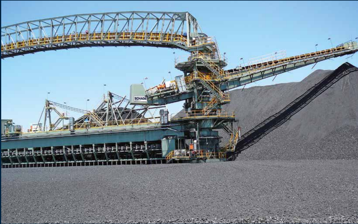
Circular Blending Bed for outdoor operation
