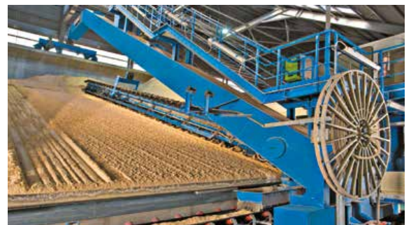
Semi-Portal Scraper Reclaimer
