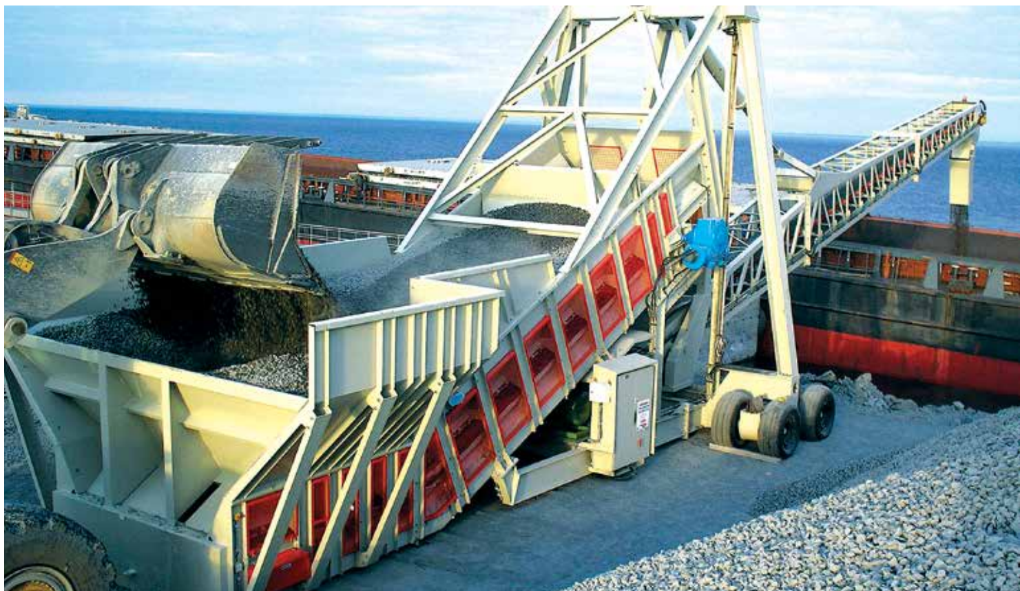
The massive Samson® MF1600 receives gabbros rock from shovels for barge loading at 1,000 t.p.h.
