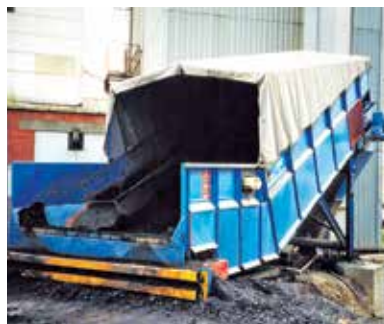
Flexible PVC sheet partial enclosure
