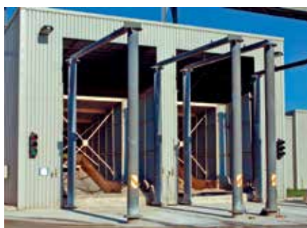
Twin Samson® Material Feeders with traffic management
