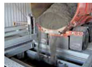
Truck discharges through open doors
