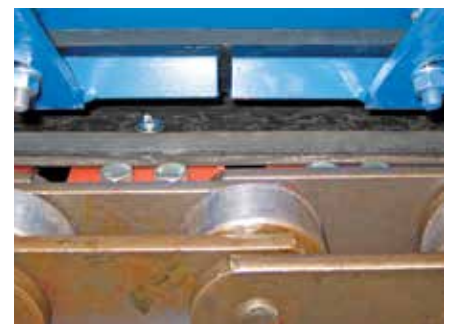
Load carried on the chain rollers
