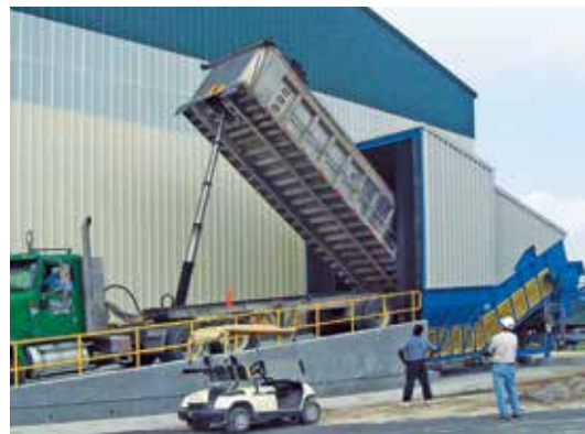
Synthetic gypsum intake to Board Plant
