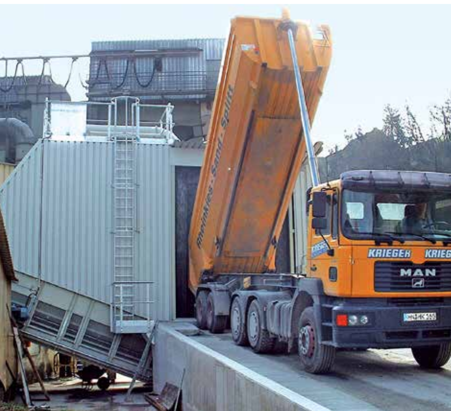
The side loading Samson® MF receives cement clinker for import directly to an existing conveyor installation
