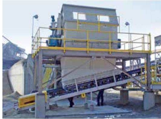
Samson® MF1600 with tandem drives using two helical/bevel speed reducers mounted one each side of the extended head shaft
