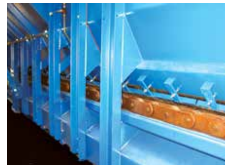
External chains outside the material flow
