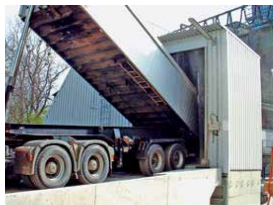
The side loading Samson® MF receives cement clinker for import directly to an existing conveyor installation
