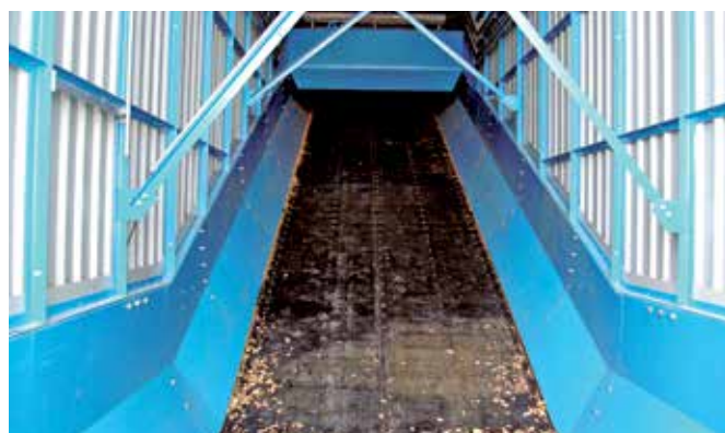
The wide apron-belt Samson® MF concept is ideal for difficult materials
