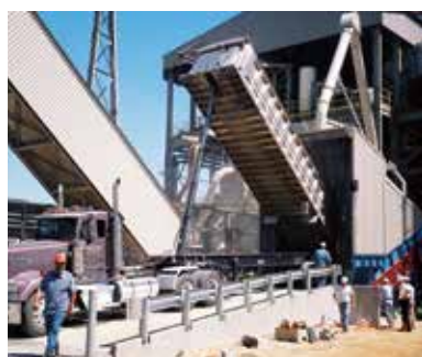
Full enclosure with ducted dust extraction
