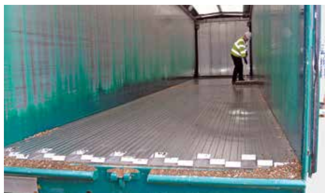
Intake from high capacity live floor trailers
