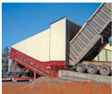
Full enclosure with flexible entry curtain but without dust extraction
