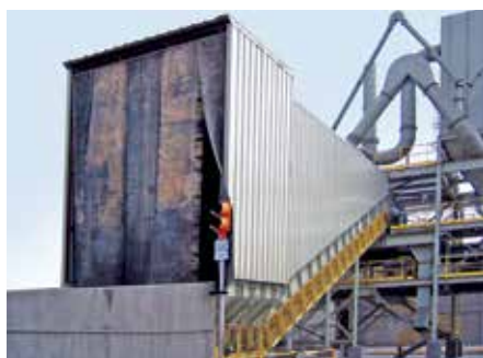
Extended inclined section for increased storage or discharge height
