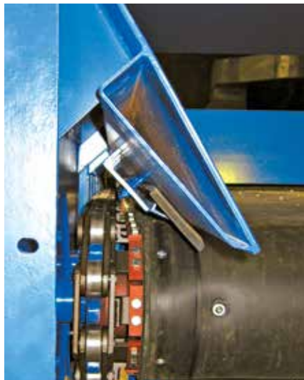
Flexible side seal with outer belt ledge
