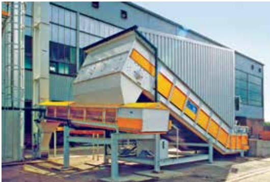
Kleen-Line belt feeder transfer to Bucket Elevator
