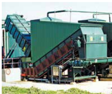
Enclosure with fume extraction for odorous materials
