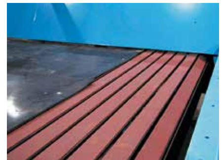
Steel apron bars support the load
