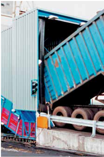
Wide belt design eliminates bridging
