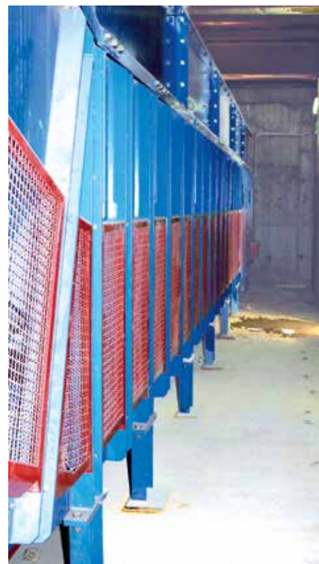
Discharge facility for hopper bottom railcars receives coal for a Cement Plant including a Samson® MF with 80 tons holding capacity
