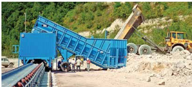
Mobile Samson® MF receives as-mined limestone from articulated trucks
