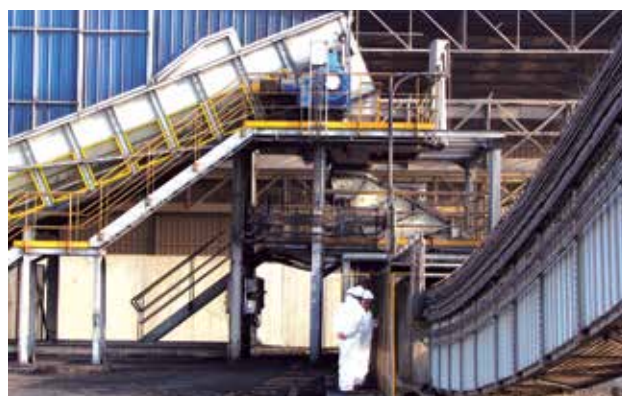
Samson® MF supplied with vibrating screen to remove oversize material before onward conveying
