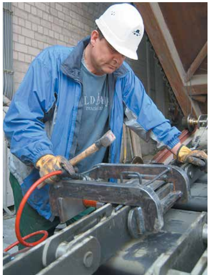
Pre-assembly of chain strands
