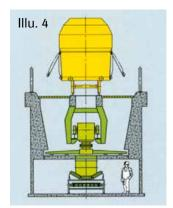
Hopper discharge with Rotary Discharge Machine type RDM
