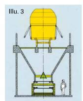
Hopper discharge with Deep-Drawn Pan Conveyor type KZB-S
