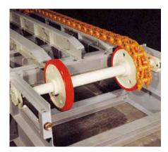
Tensioning shaft with untoothed guide wheels
