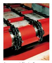
Armoured Chain Conveyor type PKF
