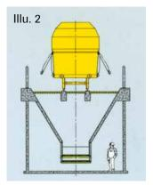
Hopper discharge with Armoured Chain Conveyor type PKF
