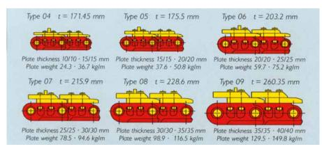
Chain-plate-combination for type BPB-S and type BPB-SF (standard) Chain size 10 and 11 on request
