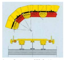
Apron Feeder type BPB-S with outboard rollers
