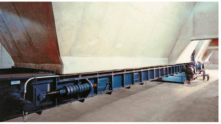
Hopper discharge with Armoured Chain Conveyor
