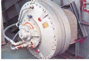
Mechanical planetary gear for type PKF
