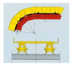
Apron Feeder type BPB-SF with stationary rollers
