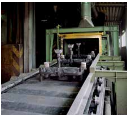
Degating with manipulator, plus cooling
