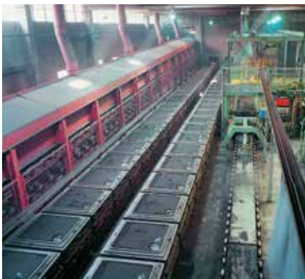
Conveying and cooling of castings
