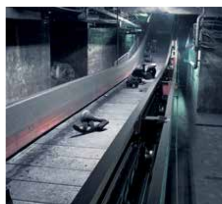
Inclined transportation of castings
