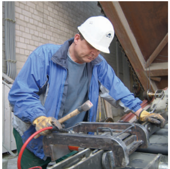
Pre-assembly of chain strands
