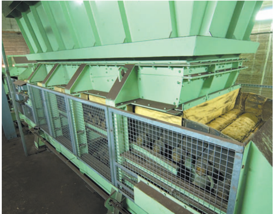
Apron Weigh Feeder with arched plates, type DPB-B Handling moist additives
