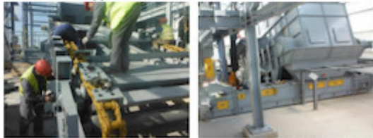
New AUMUND BPB-SLP Hybrid Feeder, a technical combination of Samson® Material Feeder and heavy-duty AUMUND BPB-SF Arched Plate Conveyor (photos AUMUND)
