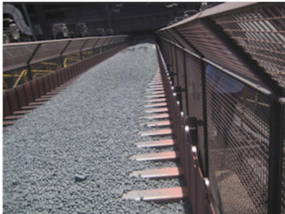
AUMUND-Pellet Conveyor type KZB (example, photo AUMUND)
