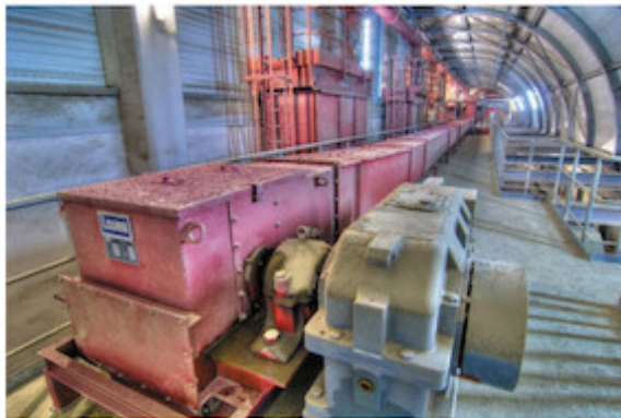
Photo1: Example of an AUMUND drag chain conveyor TKF type LOUISE (photo AUMUND)
