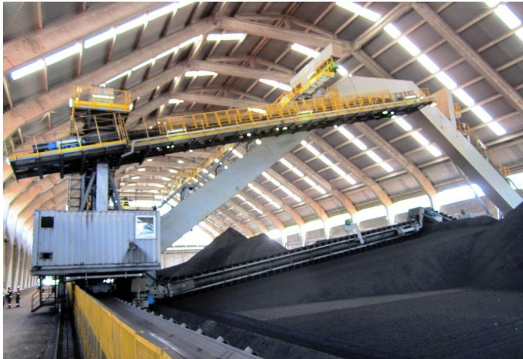
This SCHADE semi-portal reclaimer at Cerro Blanco in Ecuador is typical of those installed in China (photo SCHADE)
