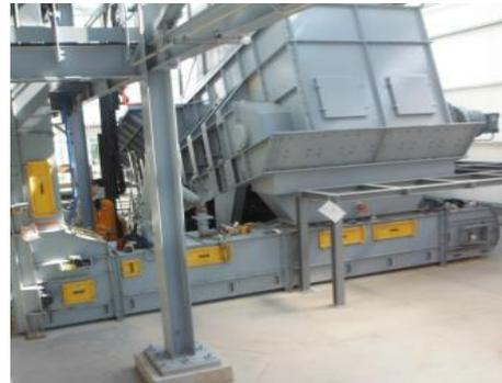
New AUMUND BPB-SLP Hybrid Feeder, a technical combination of Samson® Material Feeder and heavy-duty AUMUND BPB-SF Arched Plate Conveyor (photos AUMUND)
